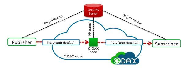
Figure 2: Content-based security for C-DAX
