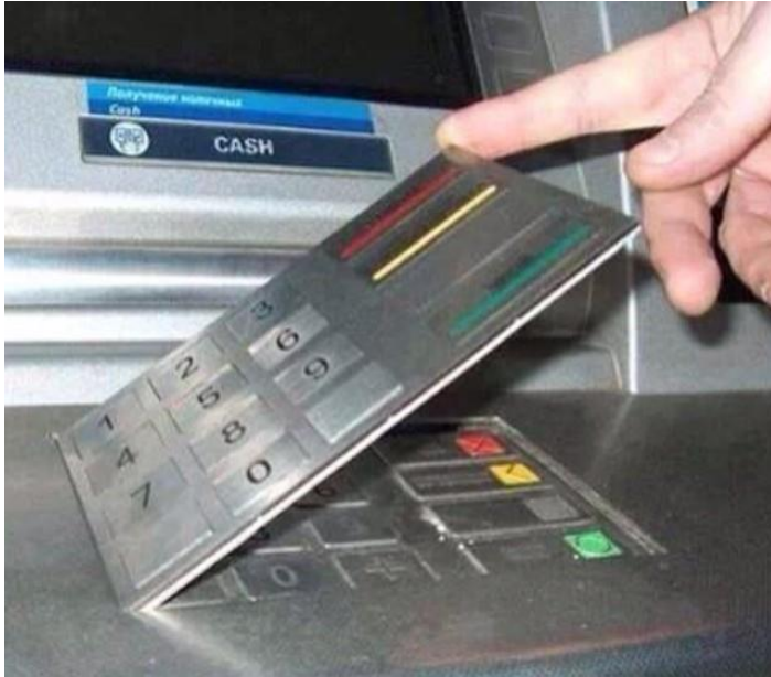
Fake keyboard to intercept PIN code
