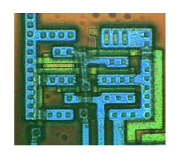
The same gate before and after etching to remove top layer
