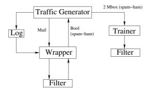
Figure 1. The design of the simulator
