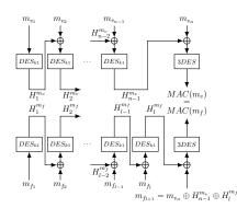
(b) Messages  $m_v$  and  $m_f$  are made to have the same MAC by adding block  $m_{f_{l+1}} = m_{v_n} \oplus H_{n-1}^{m_v} \oplus H_l^{m_f}$ .
