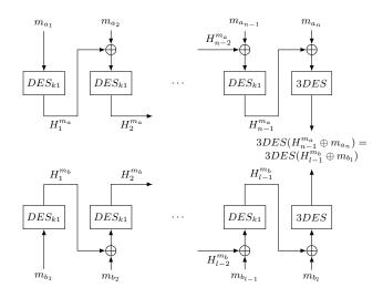
Figure 3: Recovering the DES  $k_1$  key using message collisions.
