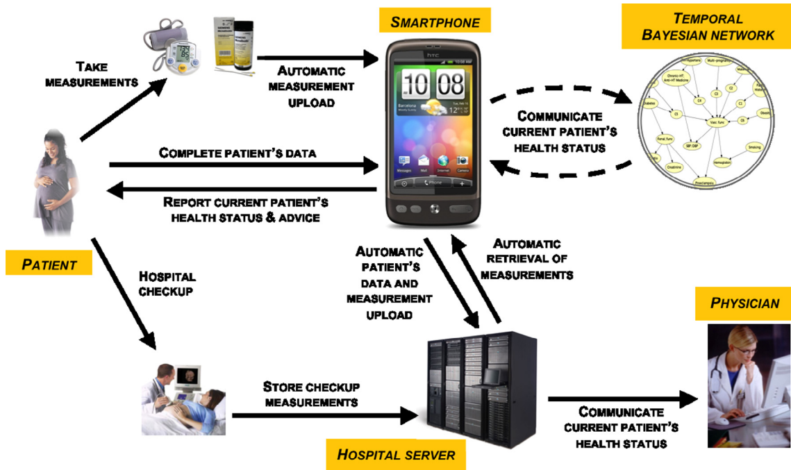
Fig. 3. Scheme of the eMomCare system's components.
