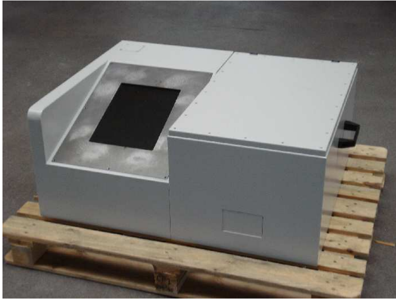
Fig. 2. A prototype tempest-shielded voteprinter, with touch screen and protected tray for the printed vote.
