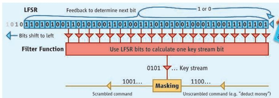
**Scramble.** As bits step through the LFSR, some feed the filter function, which makes the key stream used to scramble messages. A card's ID feeds into the LFSR, but that lets hackers control its bits.
