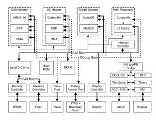
Figure 2: The ARM architecture and its AXI bus (source: [1])
