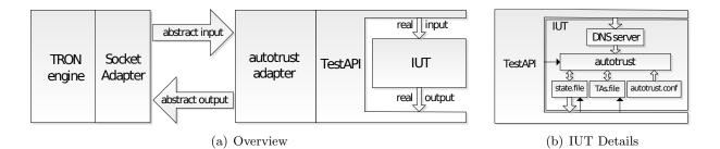
Figure 5: Specific TRON Test Setup
