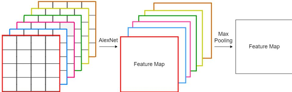
Figure 3.6: An example of Max Pooling Late Fusion. The slices are given to the feature extractor one by one. The resulting feature maps are then combined to one feature map by taking the maximum values across them.
