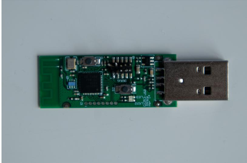
Figure 2.3: Zigbee CC2531 USB-dongle
