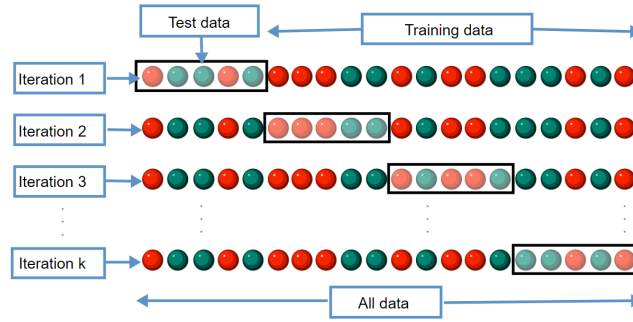
Figure 4.10: The k-fold cross-validation strategy to split data into training data and testing data.
