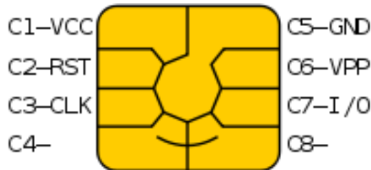
Figure 3: The pin-out scheme of a smart card. From Wikipedia/File:SmartCardPinout.svg
