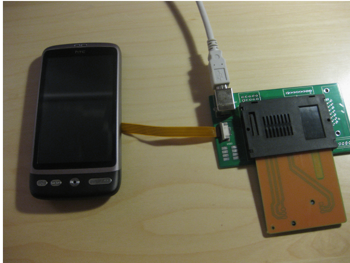
Figure 7: The RebelSIM (to the right), connected to a HTC Desire phone.
