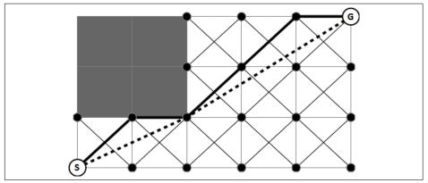
Figure 1: The grid constraint of A\*. The thick black line shows a typical A\* path from red to blue. The dotted line shows the optimal path on the continuous terrain.
