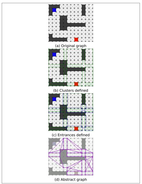
Figure 2: Process of building an abstract graph. Applies to both HPA\* and HPT\*.
