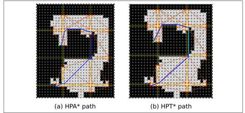
Figure 3: HPT\* versus HPA\*. During path refinement, HPA\* needs to connect all nodes on the blue path by doing A\* searches. HPT\* only needs to do a Theta\* search on the light blue line, because this is the only time the two subsequent nodes do not have line of sight.
