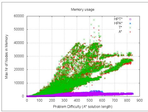
Figure 6: Maximum of nodes in memory with each algorithm.
