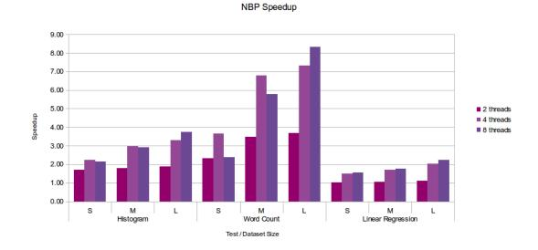
Figure 3.6: Phoenix speedups achieved on the NBP system, based on the last 10 measurements of 15 runs.
