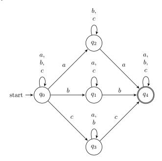
This recognises the right language because whenever a letter occurs at least two times in a word the automaton can loop in  $q_0$  until the first occurrence of the word and take the transition to another state at this first occurrence. The non-determinism is useful in this case because it allows the automaton to stay in state  $q_0$  until the letter it knows to occur twice occurs for the first time.
