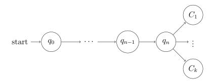
Figure 7.1: The general shape of an normal form U1NFA
