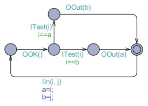
figure, a guard is added to the model. In this automaton the received input from IIn(i, j) is stored in registers a and b and the next input from ITest(i) will be compared to registers a and b. When i is equal to a, b will be the output parameter of OOut and when and i is equal to b, a will be the output parameter of OOut. Most of the time, non accepting transitions are not modelled. If i from ITest(i) is not equal to either a or b, then this automaton ends up in a non-accepting state.
