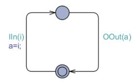
symbol starts with an I, it is considered an input. If it starts with an O, it is considered an output. Input transitions always require an input from an environment, while output transitions always follow directly after an input, as an acknowledgement.
