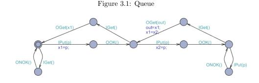
First we created three tstr objects with the strings "in1", "in2" and "in3" with taint values red, yellow and green respectively. The three tstr objects are called in1, in2 and in3. Then, the flow of inputs and outputs from Figure 3.2 were sent to and received from the state machine in Figure 3.1. The
