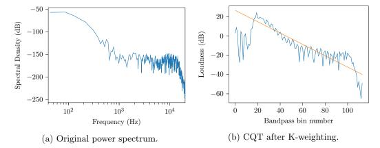
Figure 3.4: Example PSD and CQT of a kick drum sample. The linear fit has slope  $a \approx -0.587$ .
