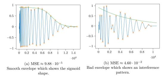
Figure 3.2: Examples of the least squares method fitting the sigmoid to a good (a) and bad (b) sample.
