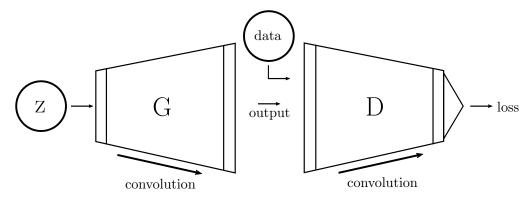
Figure 2.3: A schematic GAN architecture.
