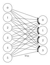
Figure 2.1: A small fully connected network. Each connection is indexed as  $w_{ij}$ , one connection is labeled as example.
