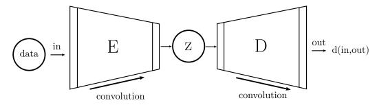
Figure 2.4: A schematic VAE architecture.
