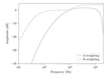
Figure 3.3: Frequency response of A-weighting and K-weighting filters.
