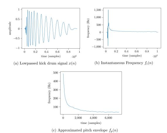
Figure 3.5: Example of finding the pitch envelope of a kick drum. This evaluates to  $f_e \approx 38.87$ , which is an Eb. Notice the IF is very inaccurate, even negative, at the very start.
