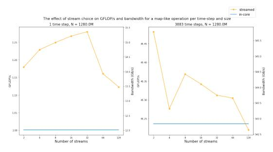
Figure 4.3: The performance of vector addition with 1280 million elements measured with different numbers of streams at 1 and 3883 time steps.
