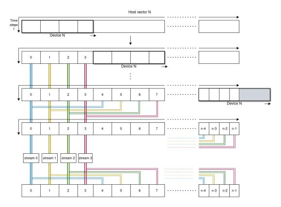
Figure 3.7: A visual representation of the device memory moving as a sliding window across the host memory.
