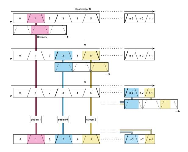
Figure 3.22: A visual representation of the device moving as a sliding window over the host in order to stream the odd trapezoids.
