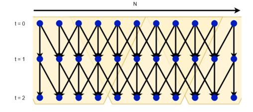
Figure 2.8: An example of overlapped tiling with stencil computations.
