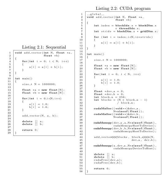
Figure 2.1: A comparison of adding two vectors in a sequential program and in a (parallel) CUDA program.
