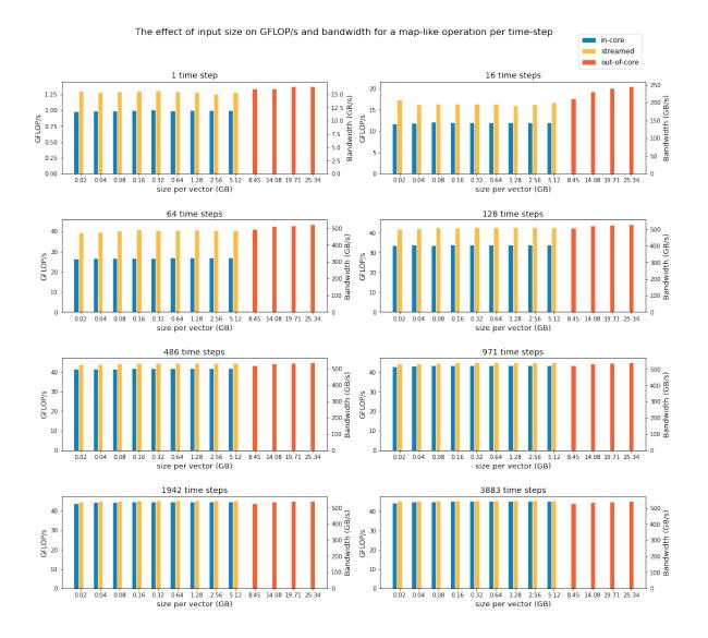
Figure 4.2: The effect of input size on the performance of an in-core, streamed and out-of-core map-like operation at all different time steps.
