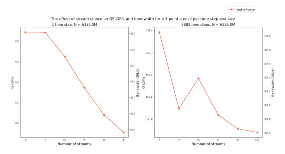
Figure 4.7: The performance of a 3-point stencil with 6338 million elements measured with different numbers of streams at 1 and 3883 time steps.
