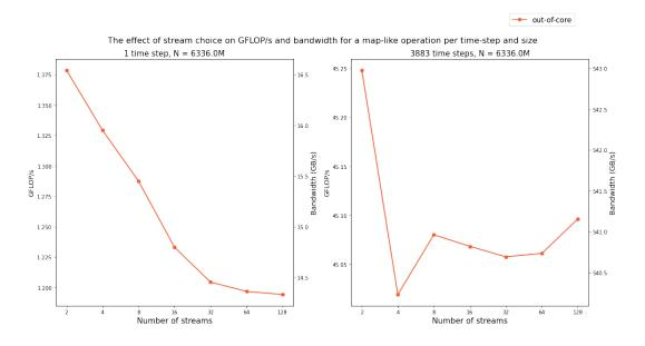
Figure 4.4: The performance of vector addition with 6338 million elements measured with different numbers of streams at 1 and 3883 time steps.
