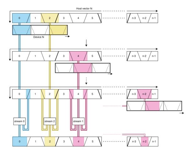
Figure 3.21: A visual representation of the device moving as a sliding window over the host in order to stream the even trapezoids.
