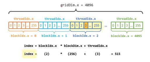
Figure 2.4: In this example, the grid contains 4096 blocks and each block has 256 threads. When the third thread in the third block of this grid executes, its corresponding index in the vector is calculated as shown. See footnote 1 for figure source.
