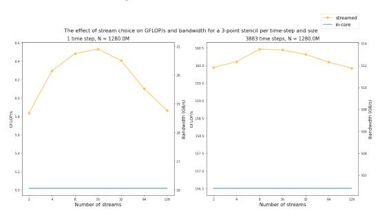
Figure 4.6: The performance of a 3-point stencil with 1280 million elements measured with different numbers of streams at 1 and 3883 time steps.
