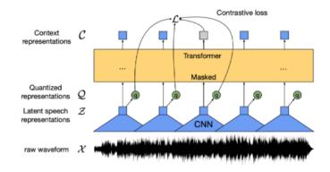
Figure 2.12: Wav2vec2 architecture [6]
