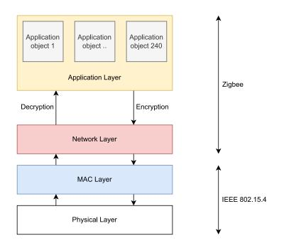
Figure 3.12: Zigbee Network Stack.
