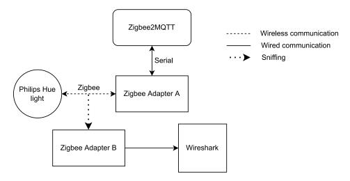
Figure 3.6: Zigbee Sniffing setup: Adapter B eavesdrops on communication between Adapter A and the Philips Hue light.
