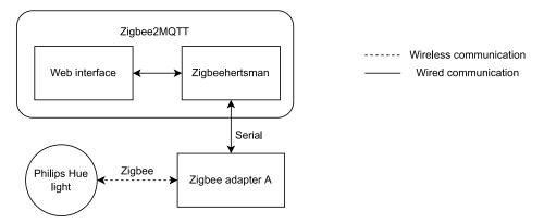
Figure 3.2: Data flow diagram for Zigbee2MQTT
