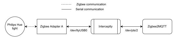
Figure 3.4: Serial port sniffing setup using Interceptty
