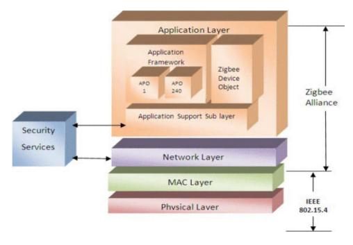
Figure 2.1: Zigbee Network Protocol Stack[17]
