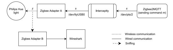
Figure 3.10: Visual representation of experiment 3.4.4, with serial frame s, Zigbee message z and Zigbee2MQTT command m.
