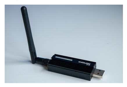
Figure 2.2: Sonoff Zigbee 3.0 USB dongle plus
