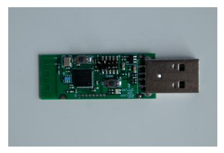
Figure 2.3: Zigbee CC2531 USB-dongle
