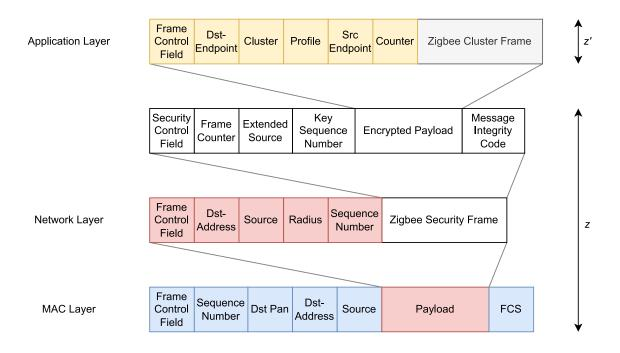
Figure 3.13: Zigbee message z split up into layers.
