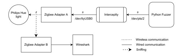
Figure 3.15: Visual representation of the fuzzing setup of the experiments in section 3.5 with serial frame s and Zigbee message z.
