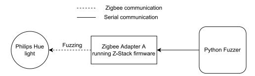
Figure 3.1: High level fuzzing setup
