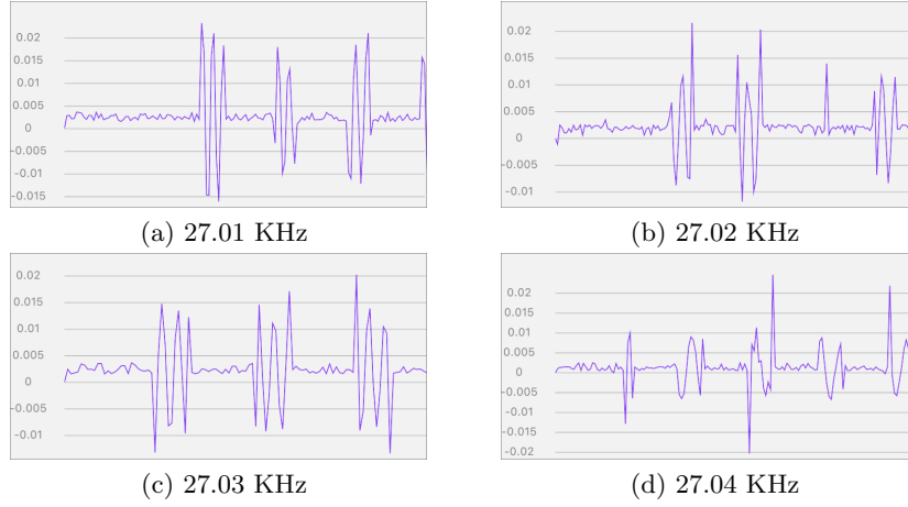
Figure 4.4: Graphs of gyroscope readings being influenced by sound waves of different frequencies
