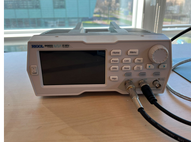
Figure 2.2: Picture of the used Rigol DG822, 2 channel oscillator
