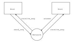
Several identical network automata in model. Each of these automata takes care of broadcasting single message (and reply) and has a clock to ensure roundtrip delay of 1sec. We assume hosts handle incoming messages instantaneously.
