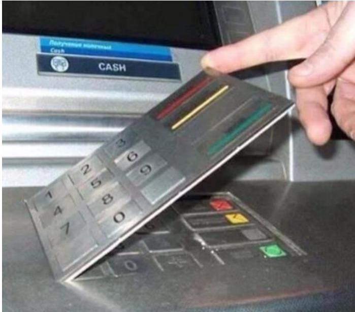
Fake keyboard to intercept PIN code
