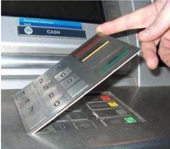
Fake keyboard to intercept PIN code
