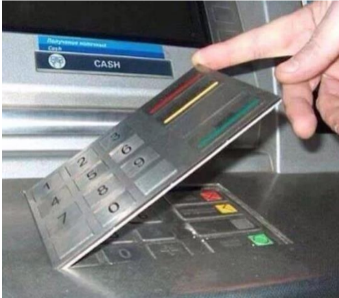
Fake keyboard to intercept PIN code
