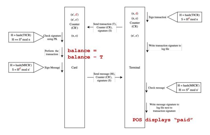
Figure 4: Signing protocol for POS terminals
