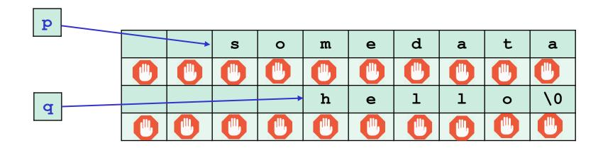
Buffer overwrite or overread will cause a memory fault.
