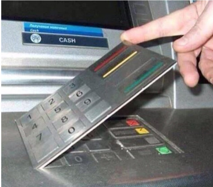
Fake keyboard to intercept PIN code
