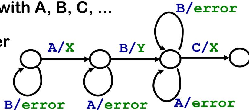
The inferred state machine is **under-approximation** of real system
