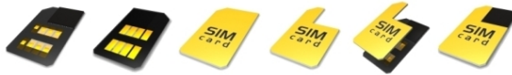
Figure 2.7: Picture from the Bladox website [18] showing how to cut the SIM card to place the Turbo SIM in between SIM and phone.
