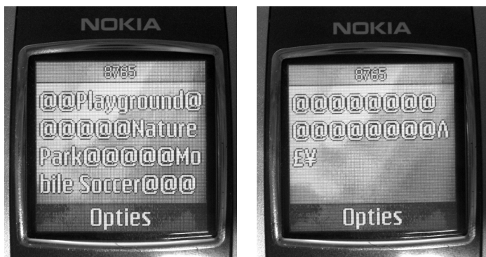
Figure 6.6: These two pictures show the strange behaviour when the same SMS is opened twice in a row. Note that the words in the left image are the names of games available on the device.
