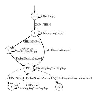
Fig. 5. State machine of an OpenVPN or OpenVPN-NL server running in UDP mode.
