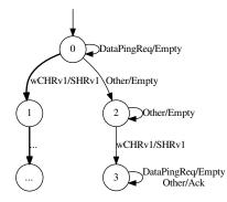
Fig. 7. Subset of the state machine of an OpenVPN or OpenVPN-NL server, focusing on the particularity of the UDP mode. State 1 and its subsequent states are identical to the TCP version.
