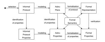
Figure 1. The process of guideline formalisation and verification as done in the Protocure project.
