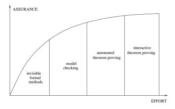
**Figure 12.** A spectrum of formal methods for formal verification allowing a tradeoff in the properties one can verify (assurance dimension) against the effort one needs to invest to obtain results (effort dimension).
