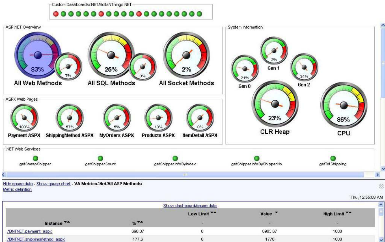
Figure 5: The Vantage Web Services Dashboard provides a user-customizable interface to monitor the overall health of an application. It can be made up of one or more gauges based on user-selected metrics, such as WMI and/or method-level data.
