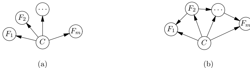
Figure 4: A naïve Bayesian network, (a), and a tree-augmented Bayesian network, (b); the nodes F_j indicate the feature variables and C is the class variable.
