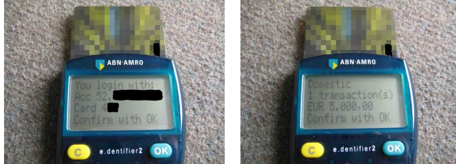
Fig. 1. The USB-connected reader, with the bank card sticking out the top, showing transaction details for the user to approve a login (left) or a bank transfer (right).
