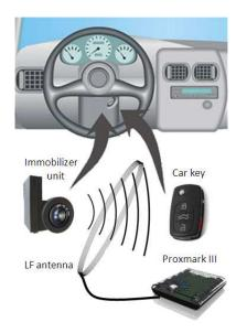
Figure 5: Experimental setup for eavesdropping
