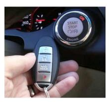
Figure 3: Keyless hybrid transponder and engine start/stop button
