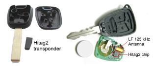
Figure 1: Car keys with a Hitag2 transponder/chip
