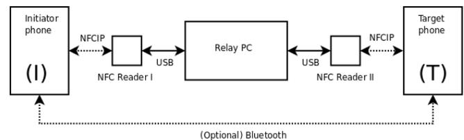
Fig. 2: NFCIP Relay Design
