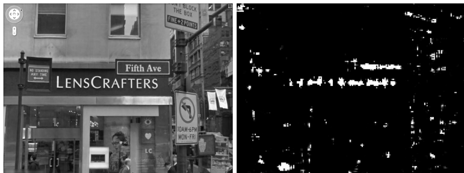
Figure 3.3: An image from Street View Text dataset at scale 0.6 and the corresponding detector response map at scale 0.6. White parts in the response map indicate the presence of text.
