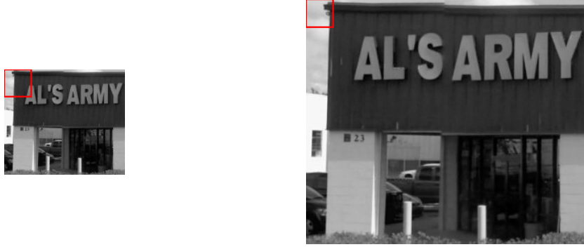
Figure 3.1: Part of an image from the Street View Text dataset [20] on the left at scale 0.3 and on the right at 0.7. The red square in the top-left corner is the window of 32 by 32 pixels. On the left, using scale 0.3, the individual characters on the storefront fit into the window. At scale 0.7 the characters do not fit into the window.
