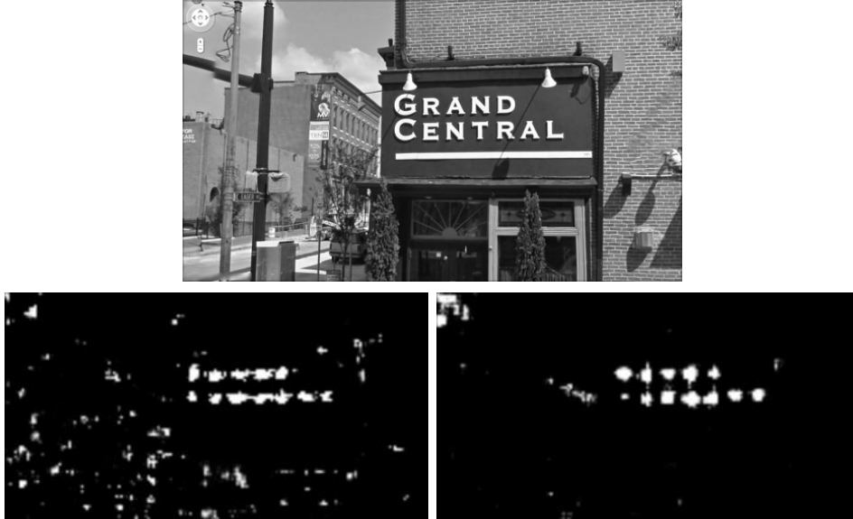
Figure 3.9: An image from the Street View Text dataset, the response map using a CNN and using ResNet-20 (20 layers; 3 residual blocks) at scale 0.4.
