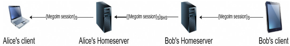
Figure 4.4: Schematic diagram of the encrypted and signed Megolm session
