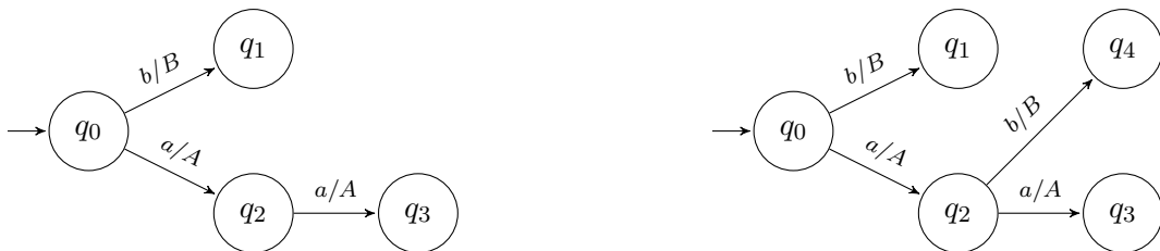
Figure 3.1: An observation tree (left) and a possible extension (right).
