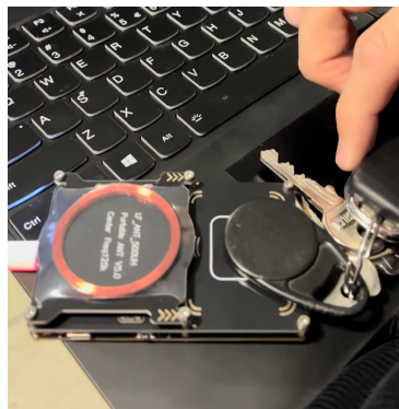
Figure 20: The tag on the ProxMark3
