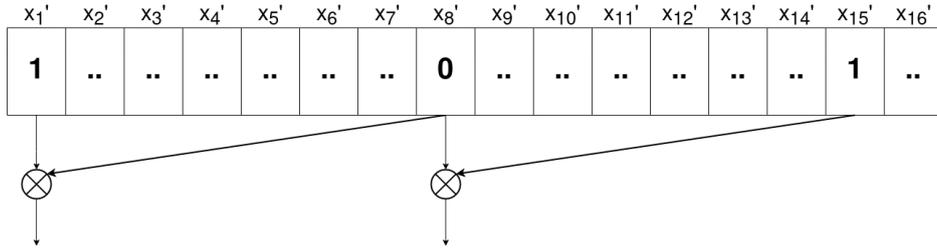
If bit  $x_1 = x_{15} = 1$  and bit  $x_8 = 0$ . The probability that both ANDs in Figure 5.2 will result in 0, is  $\frac{1}{2}$ , just as explained earlier for Figure 5.1.
