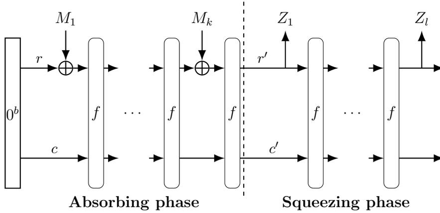
Figure 2.1: Generalized sponge construction as described in Section 2.1.
