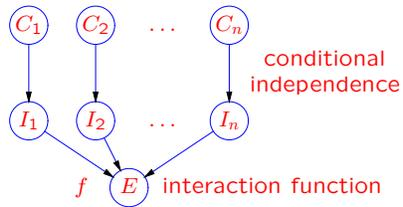
$$\begin{aligned} \Pr(e | C_1, \dots, C_n) &= \sum_{I_1, \dots, I_n} \Pr(e | I_1, \dots, I_n) \prod_{k=1}^n \Pr(I_k | C_k) \\ &= \sum_{f(I_1, \dots, I_n) = e} \prod_{k=1}^n \Pr(I_k | C_k) \end{aligned}$$
