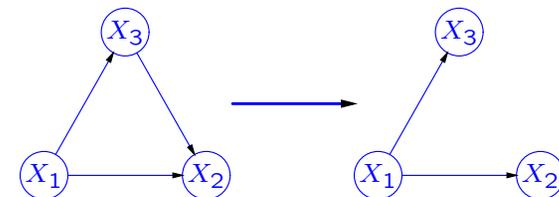
Only  $5 = 2 + 2 + 1$  probabilities needed for  $\text{Pr}(X_1, X_2, X_3)$  (instead of 7)
