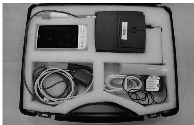
Fig. 2. The monitoring kit consisting of a smartphone, sensor interface and sensors.
