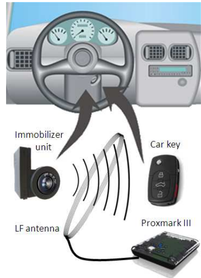
Figure 7.4: Experimental setup for eavesdropping
