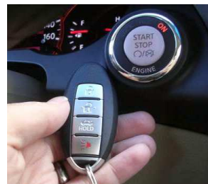
Figure 7.3: Keyless hybrid transponder and engine start/stop button
